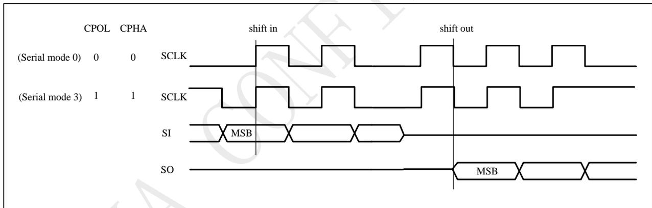
Note: CPOL indicates clock polarity of serial master, CPOL=1 for SCLK high while idle, CPOL=0 for SCLK low while not transmitting. CPHA indicates clock phase. The combination of CPOL bit and CPHA bit decides which serial mode is supported.
