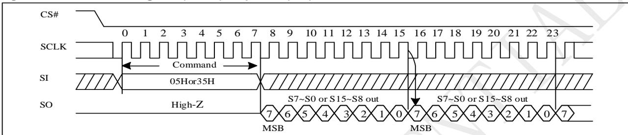
**Figure 9-5a Read Status Register (RDSR) Sequence (QPI)**
