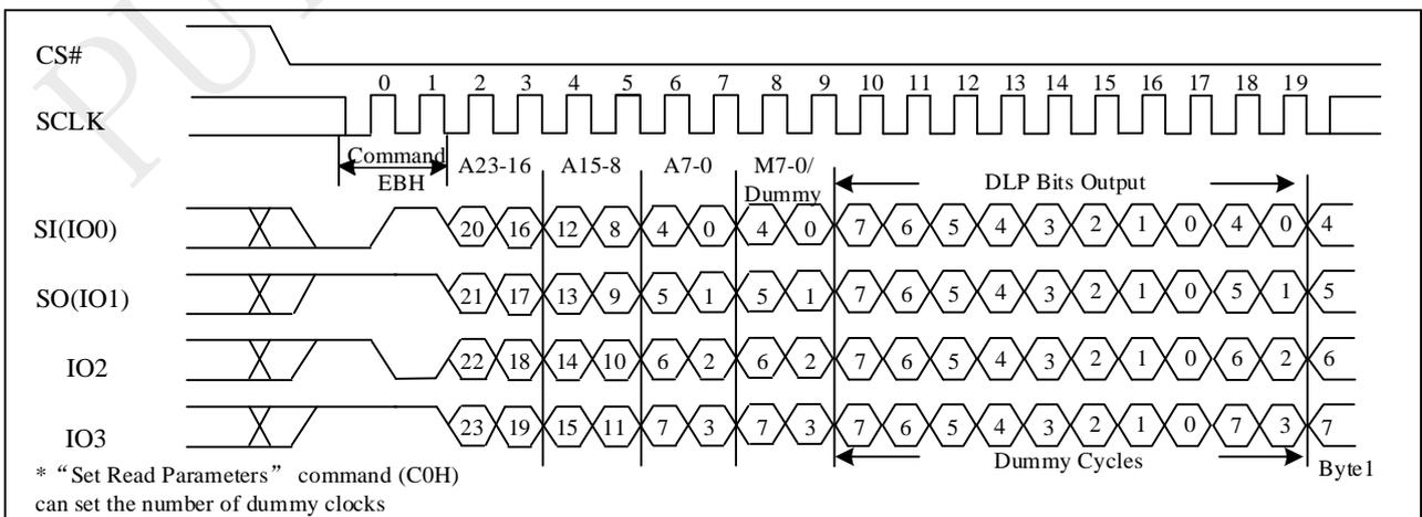
**Figure 9-30g DTR 1IO Read with DLP bits output Sequence (SPI)**
