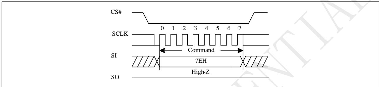
**Figure 9-62a Global Block Lock (QPI)**
