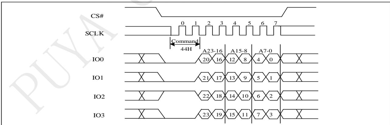
Note: 32-bit address is required when the device is operation in 4-Byte Address Mode.
