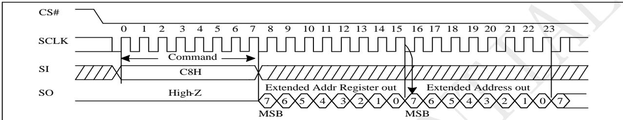
Figure 9-9a Read Extended Address Register Sequence (QPI)
