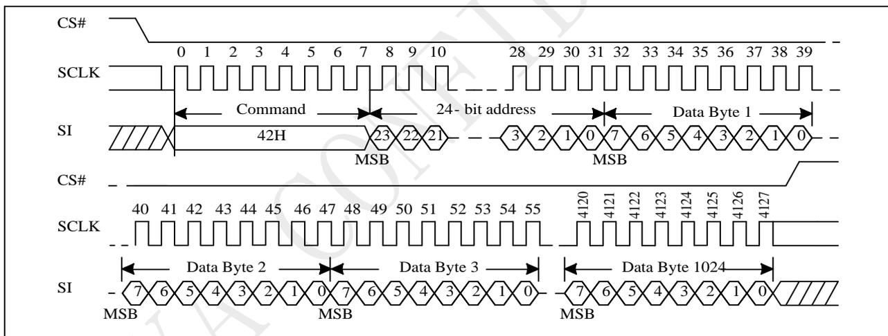
Figure 9-47a Program Security Registers (PRSCUR) Sequence (QPI)
