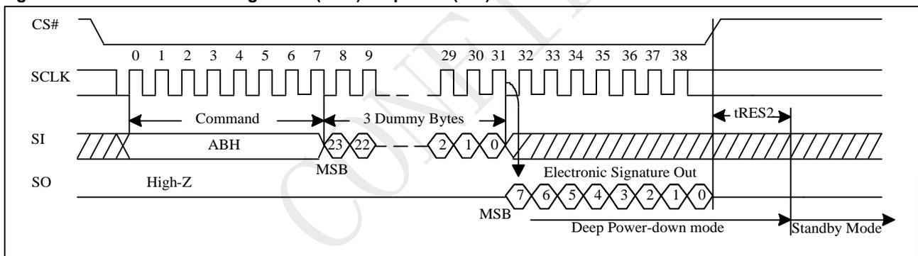
**Figure 9-50a Read Electronic Signature (RES) Sequence (QPI)**
