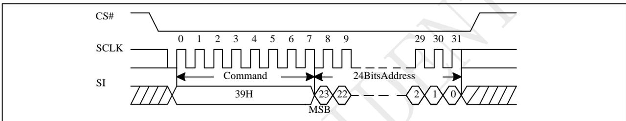
Note: 32-bit address is required when the device is operation in 4-byte address mode.
