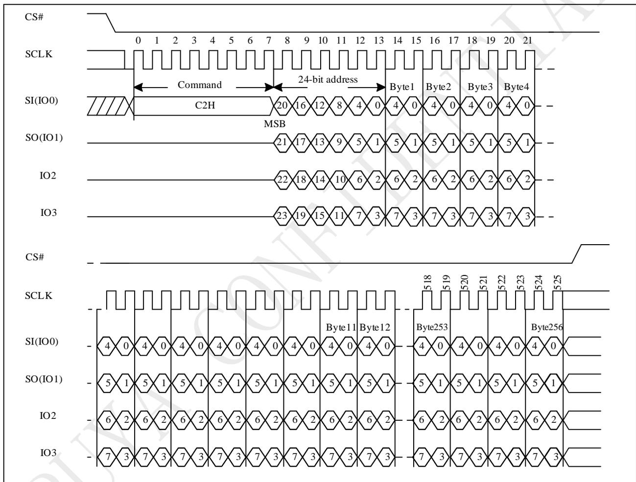
Note: 32-bit address is required when the device is operation in 4-Byte Address Mode.
