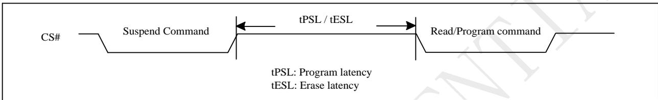
**Figure 9-56a Suspend to Read/Program Latency(QPI)**
