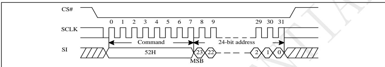
Note:32-bit address is required when the device is operation in 4-Byte Address Mode.
