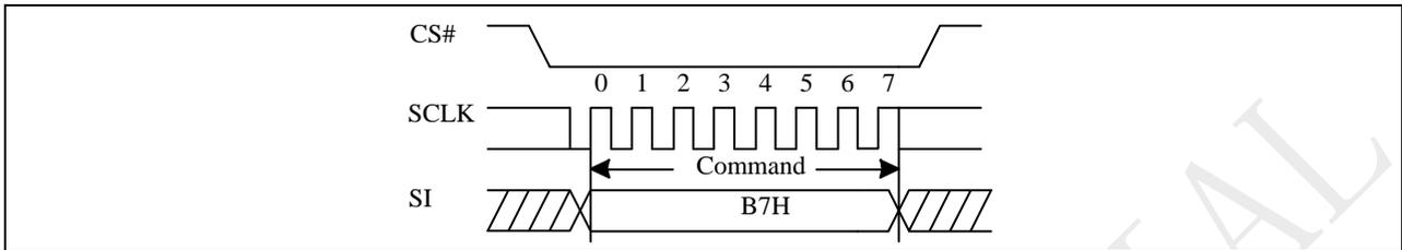
**Figure 9-11a Enter 4-Byte Address Mode Sequence (QPI)**
