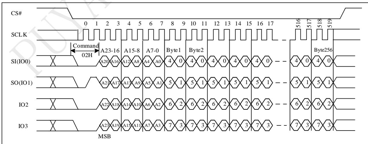
Note: 32-bit address is required when the device is operation in 4-Byte Address Mode.
