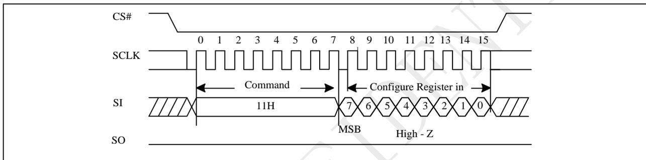
**Figure 9-8a Write Configure Register (WRCR) Sequence (QPI)**
