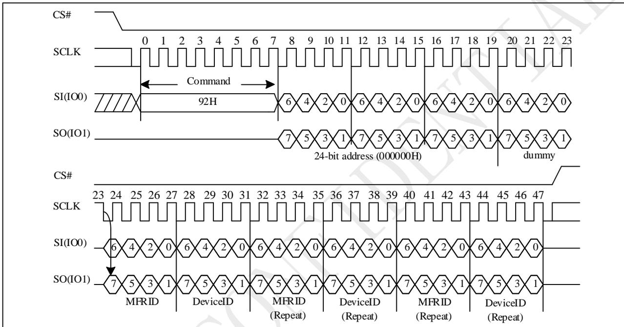
Note: 32-bit address (0000\_0000H) are required when the device is operation in 4-Byte Address Mode.
