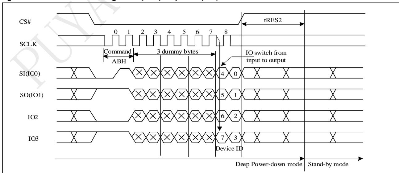
**Figure 9-50b Release from Deep Power-down (RDP) Sequence (SPI)**
