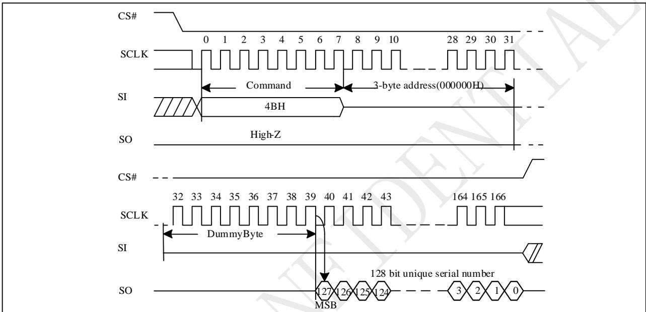
Note: 4 bytes address 0000\_0000H is required when the device is operation in 4-Byte Address Mode.
