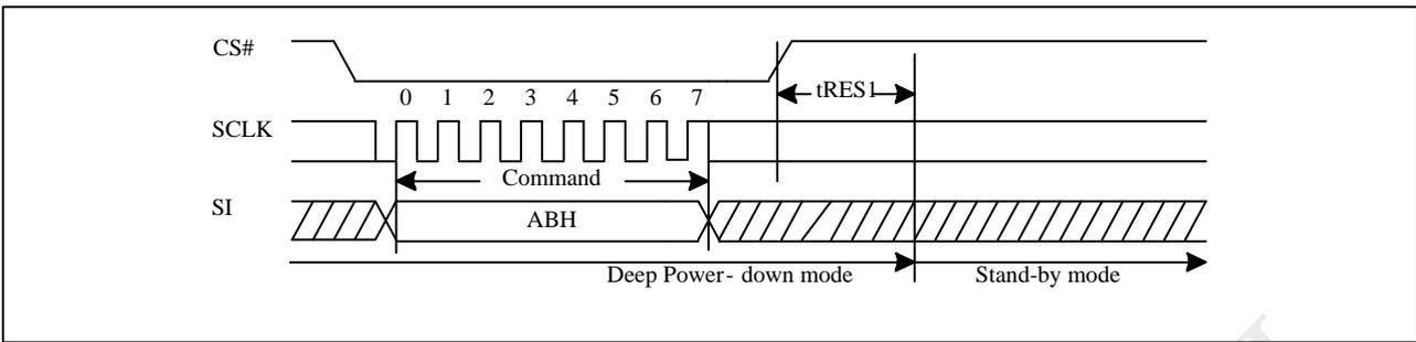
**Figure 9-50c Release from Deep Power-down (RDP) Sequence (QPI)**
