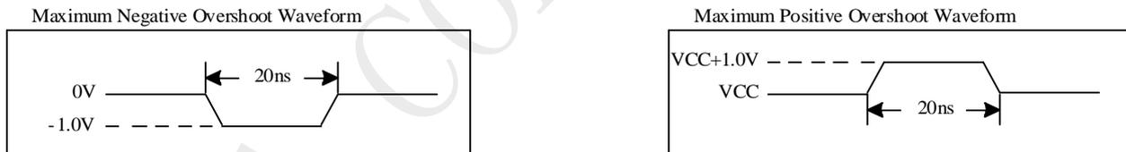
During DC conditions, input or I/O signals should remain equal to or between VSS and VCC. During voltage transitions, inputs or I/Os may negative overshoot to -1.0V or positive overshoot to VCC + 1.0 V, for periods up to 20 ns.
