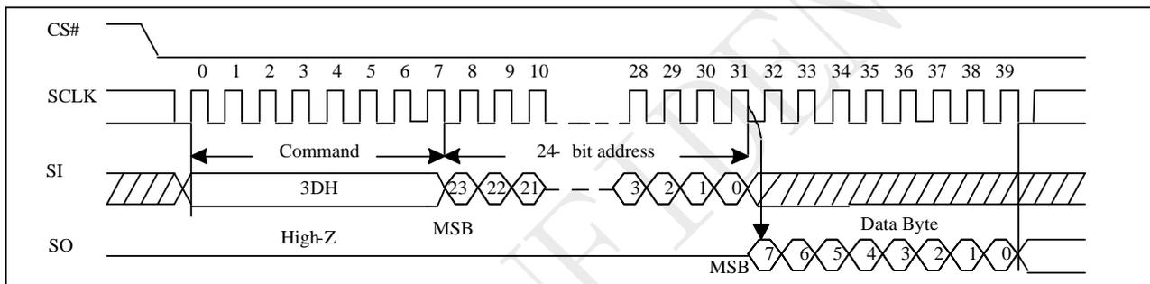
Note: 32-bit address is required when the device is operation in 4-Byte Address Mode.
