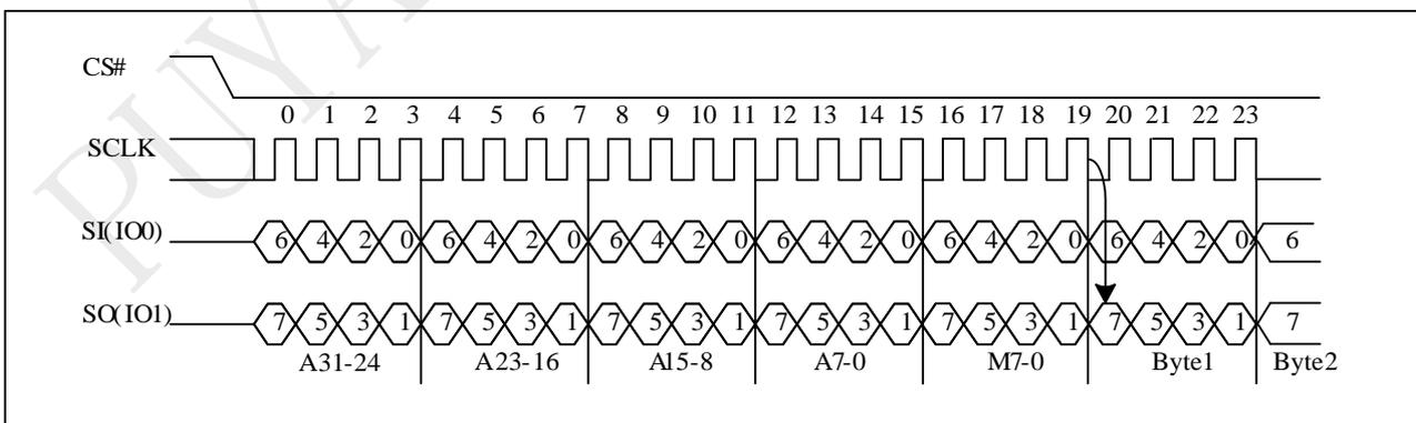
Note: 2IO Continue Read with 4-Byte Address, if M5-4 = 1, 0. If not using Continue Read recommend to set M5-4 ≠ 1, 0.
