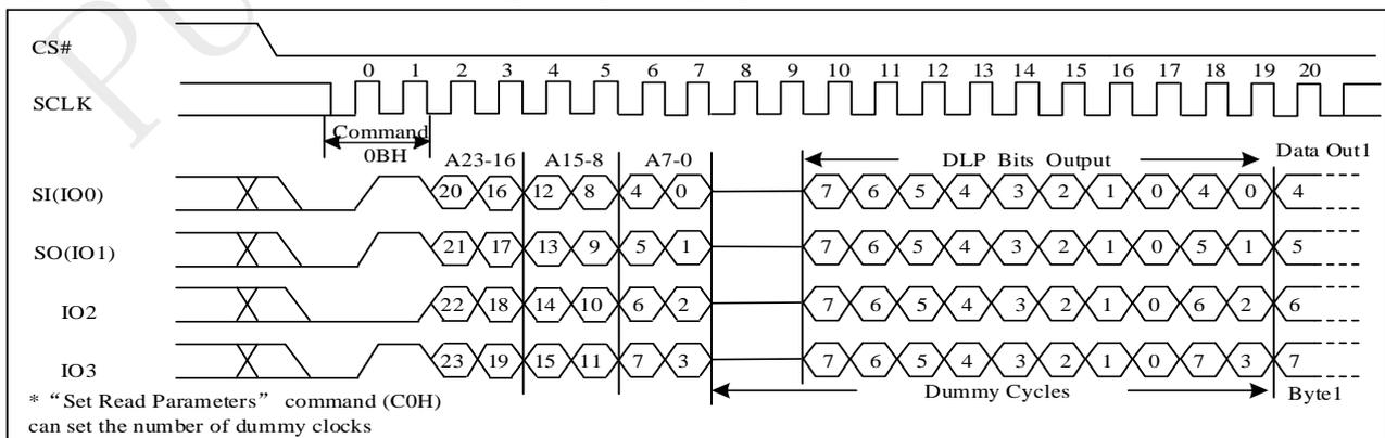
**Figure 9-30b Dual Read with DLP bits output Sequence (SPI)**
